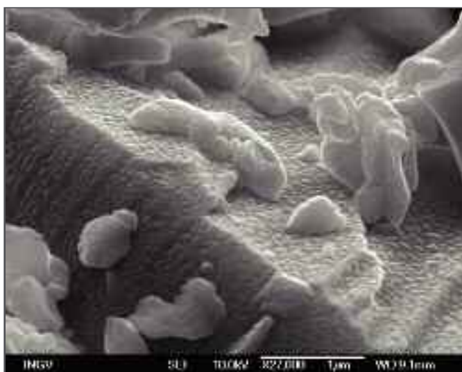
Fig. 1 | The anhydrite coating of volcanic glass particles exposed to \text{SO}_2 in the Advanced Gas-Ash Reactor (AGAR) at University of Munich, Germany.
