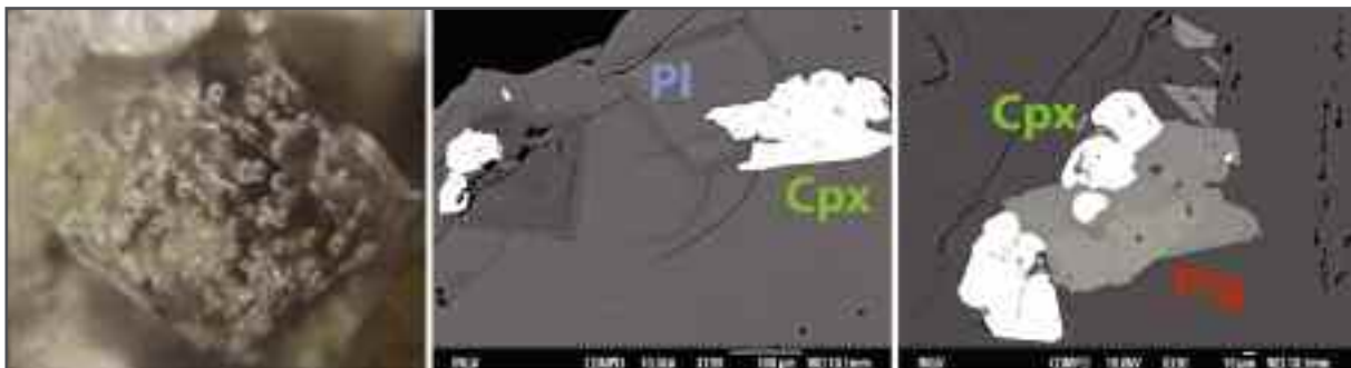
Fig. 1 | Microscope (left) and backscattered electron (centre-right) images of the rhyolitic fragments collected at the IDDP-1. Legend: plagioclase (Pl), augite (Cpx), pigeonite (Pig).
