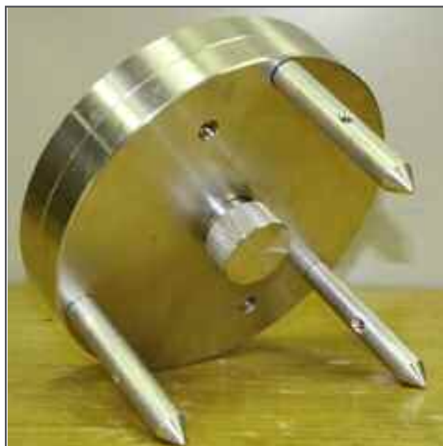
Fig. 2 | Amagnetic pedestal for declination-inclination magnetometers.
